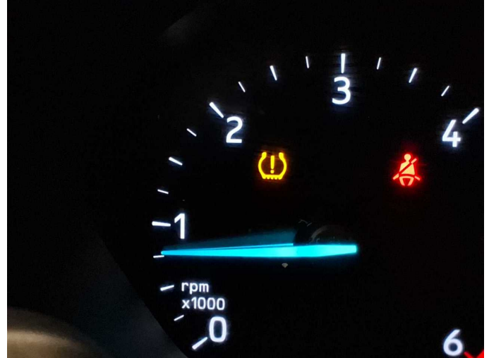
Damage 4: Instrument panel: Indicator light (Reifendruck) - on - Perform diagnosis
