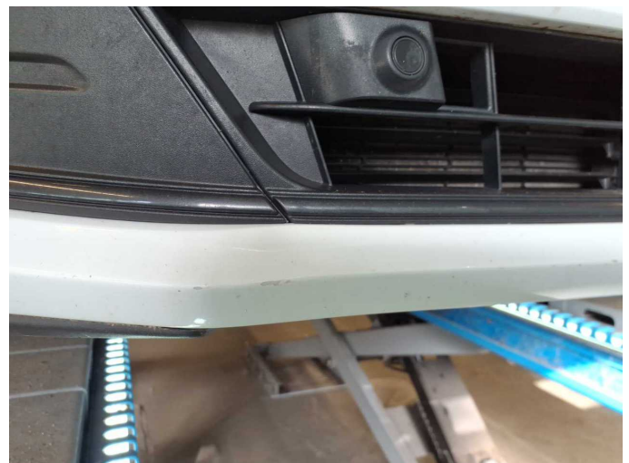
Damage 5: Front bumper: Front bumper - Scratch(es) - Paint
