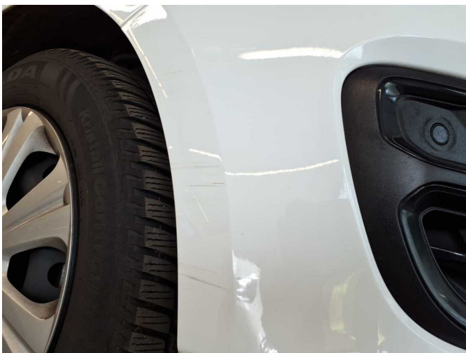
Damage 5: Front bumper: Front bumper - Scratch(es) - Paint
