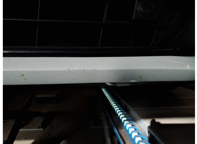
Damage 5: Front bumper: Front bumper - Scratch(es) - Paint
