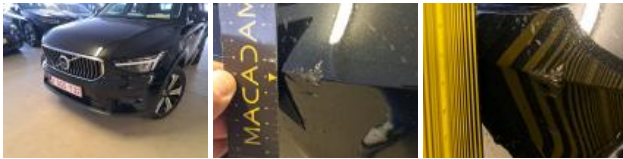
Bonnet, Bad repair, Repair and paint (complete)
