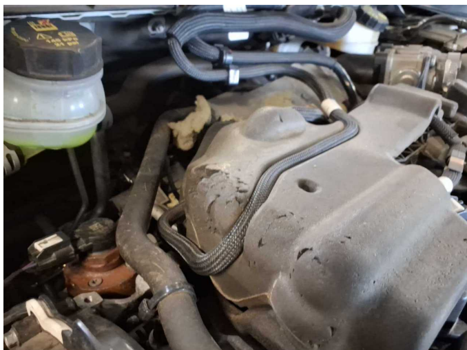
Damage 2: Engine: Engine cover (Dämmung) - Damage caused by marten / rodent - Replace
