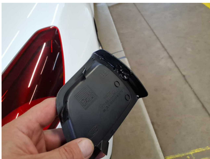
Damage 1: Trim / covers: Boot lid - interior trim - Loose - Replace
