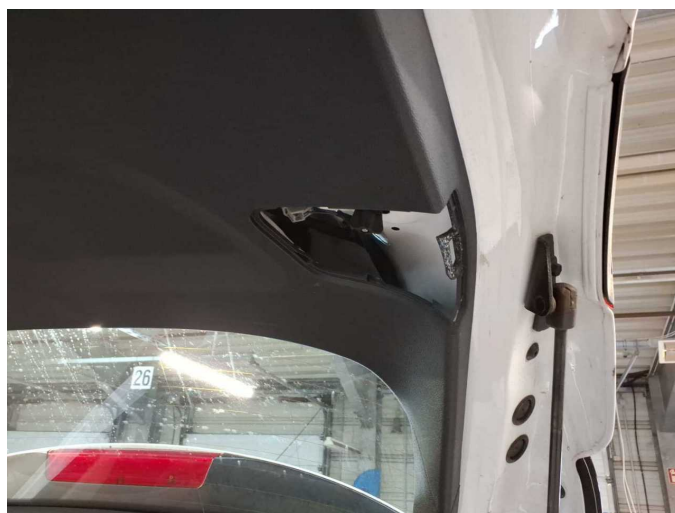
Damage 1: Trim / covers: Boot lid - interior trim - Loose - Replace
