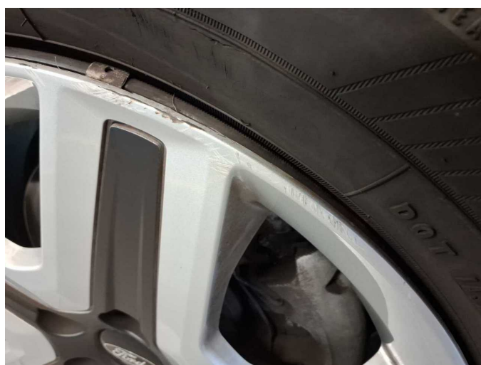
Wear and tear 4: Wheel / tyres: Wheel cover - front right side - Scratch(es) - No deduction
