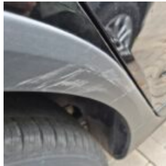
Damage Type Scratch(es)
