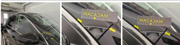
Side window trim FR, Scratch(es), Replace
