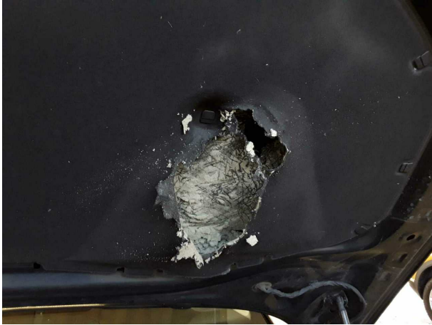
Damage #3: Bonnet: Insulation lining - Damage caused by marte... rodent - Replace
