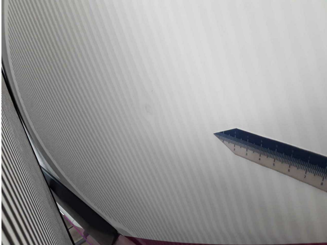
Damage 3: Side panel - rear left side: Side panel - Deformed - Smooth repair work
