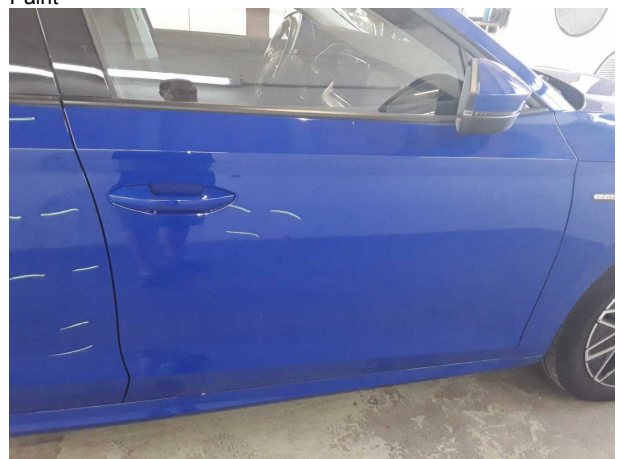
Damage #7: Door - front right side: Door - Scratched - Paint
