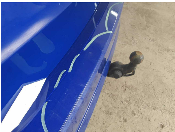
Damage #2: Rear bumper: Rear bumper - Scratched - Paint
