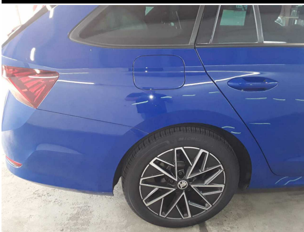
Damage #5: Side panel - rear right side: Side panel - Scratched - Paint
