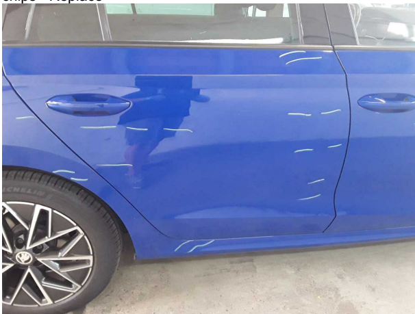
Damage #4: Door - rear right side: Door - Scratched - Paint
