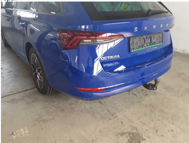
Damage #2: Rear bumper: Rear bumper - Scratched - Paint
