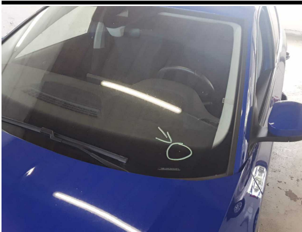
Damage #3: Vehicle glazing: Windscreen (Rissbildung) - Stone chips - Replace
