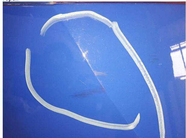
Damage #2: Rear bumper: Rear bumper - Scratched - Paint
