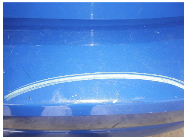
Damage #2: Rear bumper: Rear bumper - Scratched - Paint
