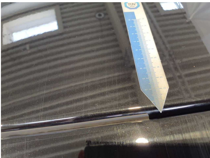
Damage 19: Roof: Roof (+ Relling li. erneuern) - Scratch(es) - Paint
