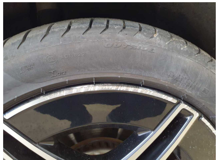
Damage 16: Wheel / tyres: Alloy rim - rear right side - Scratched - Replace
