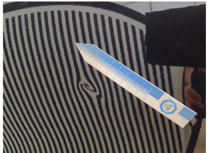
Damage 12: Door - rear left side: Door - Deformed - Repair and paint
