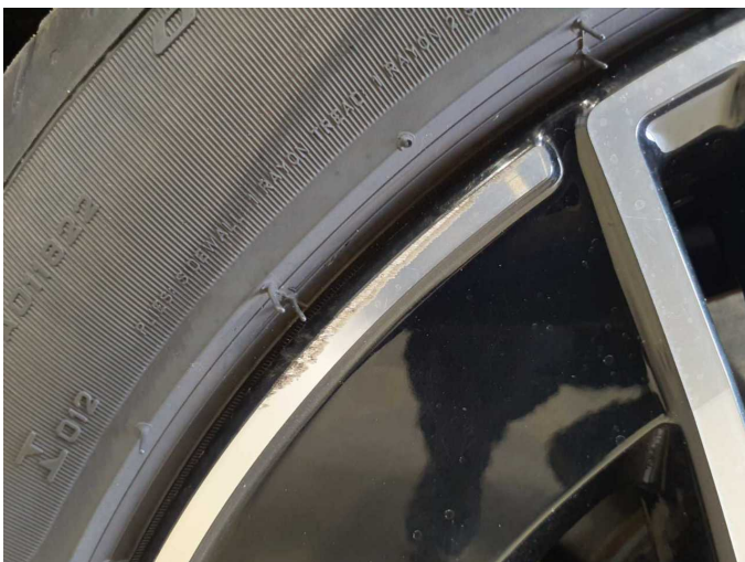
Damage 10: Wheel / tyres: Alloy rim - rear left side - Scratch(es) - Loss in value
