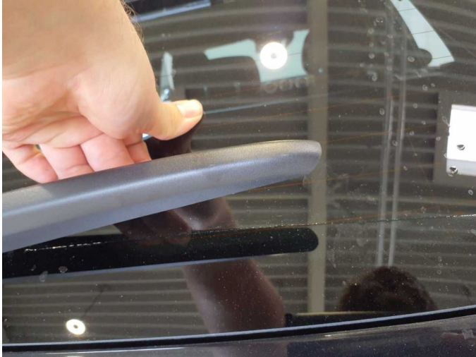
Damage 3: Screen cleaning: Wiper blades - rear - Broken / torn - Replace
