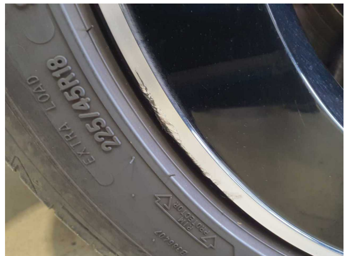
Damage 15: Wheel / tyres: Alloy rim - front left side - Scratched - Replace
