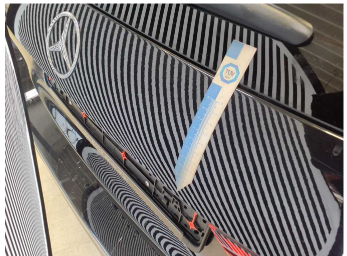
Damage 5: Boot lid / rear door: Boot lid - dent(s) - Smooth repair work
