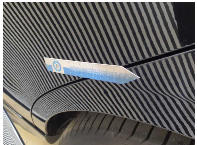
Damage 17: Side panel - rear left side: Side panel - Dent / paintcoat damage - Repair and paint
