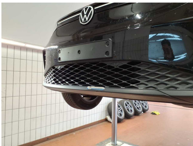
Damage 7: Front bumper: Spoiler - Scratched - Replace
