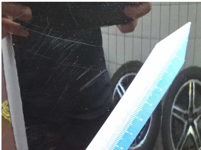
Damage 8: Rear bumper: Rear bumper (Hinten Rechts) - Scratch(es) - Paint
