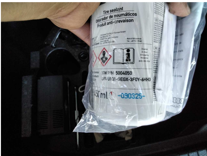
Damage 2: Equipment: Tirefit filler - Expired - Replace
