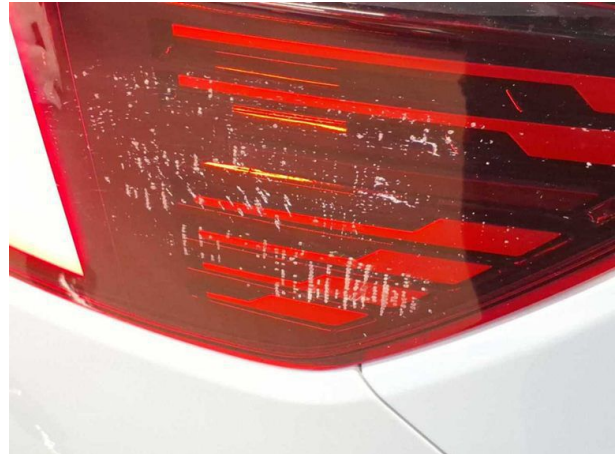
Damage #1: Tail light: Tail lamp - right side (Klebereste) - Glued / labelled - Clean
