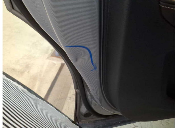
Beschädigung #2: Tür hinten links: Tür - Delle / Lackschade... Smart Repair
