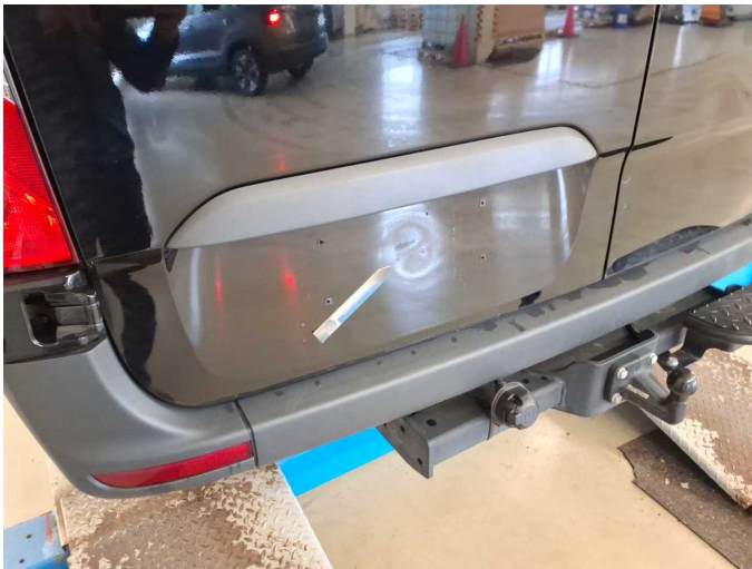
Damage 4: Boot lid / rear door: Rear door - left side - dent(s) - Repair and paint
