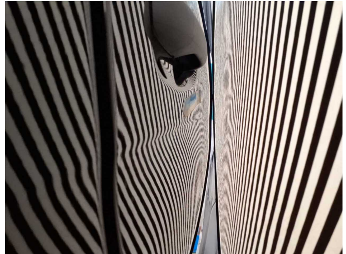
Damage 3: Door - front right side: Door - dent(s) - Smart repair
