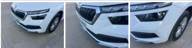
Bumper F, Scratch(es), Repair and paint (complete)
