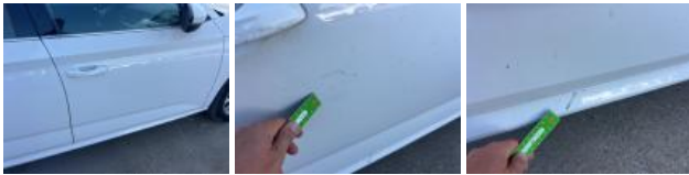
Door RR, Scratch(es), Repair and paint (complete)
