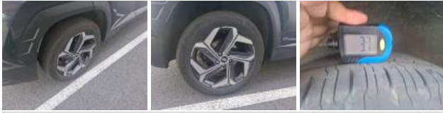
Tyre FL, Out of tolerance, Replace
