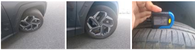
Tyre RR, Out of tolerance, Replace
