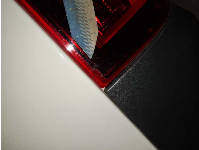
Damage 9: Tail light: Tail lamp - left side - Broken / torn - Replace
