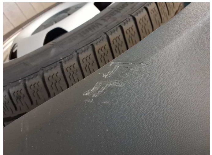
Damage 7: Front bumper: Front bumper (unpainted) - Scratch(es) - Smart repair
