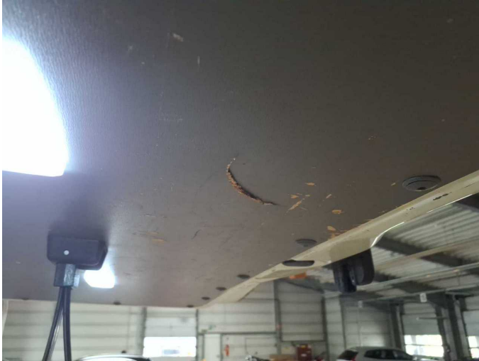
Damage 5: Trim / covers: Boot lid - interior trim - Broken / torn - Replace
