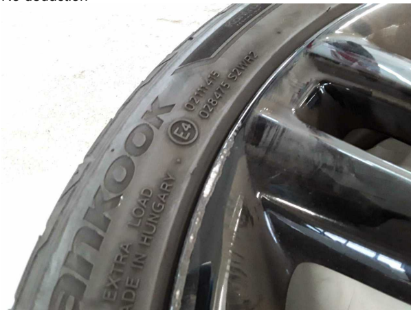
Damage #2: 2nd wheel set: 1 alloy rim - Scratched - Loss in value
