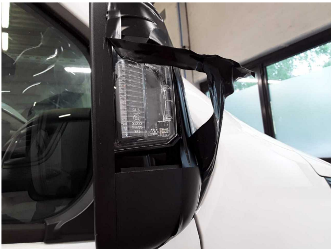
Damage 2: Wing mirror - right side: Mirror housing - Damaged - Replace
