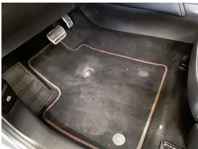
Damage 1: Trim / covers: Floor mats - Damaged - Replace
