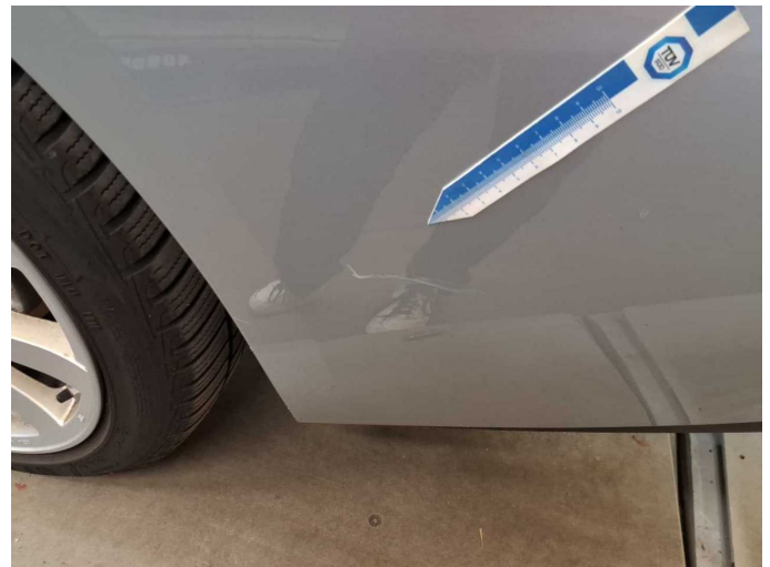
Damage 5: Rear bumper: Rear bumper - Scratch(es) - Paint
