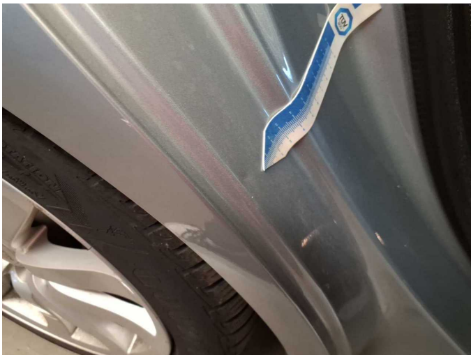
Damage 3: Side panel - rear right side: Sill - dent(s) - Smooth repair work
