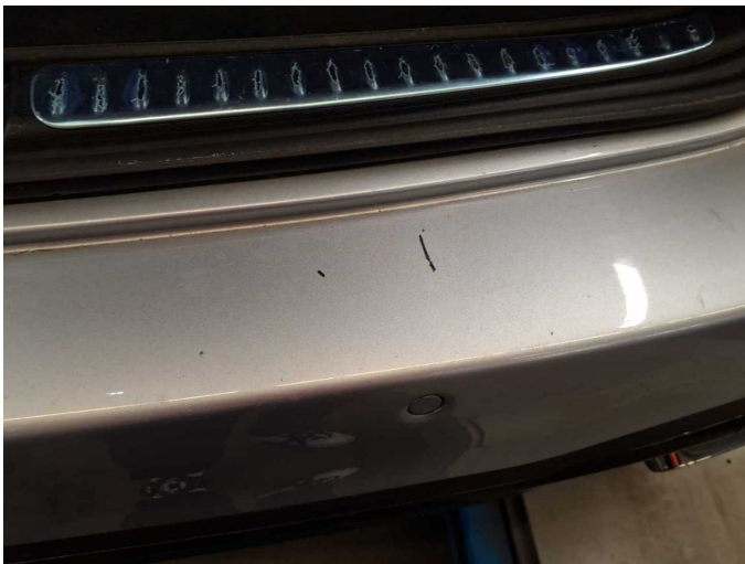
Damage 5: Rear bumper: Rear bumper - Scratch(es) - Paint
