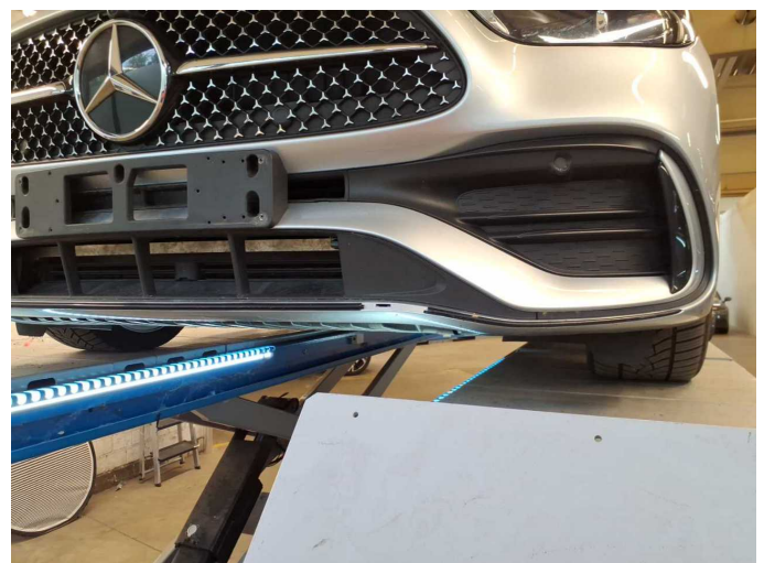
Damage 2: Front bumper: Front bumper (Zierleiste) - Broken / torn - Replace
