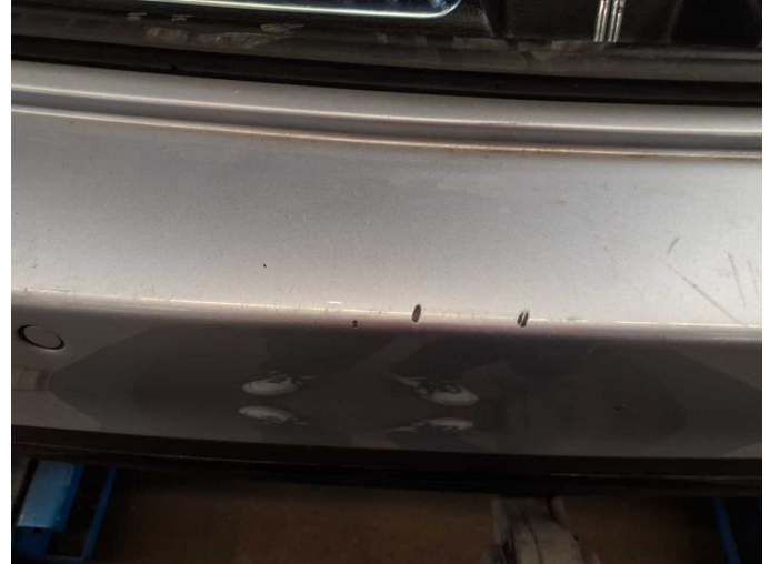
Damage 5: Rear bumper: Rear bumper - Scratch(es) - Paint
