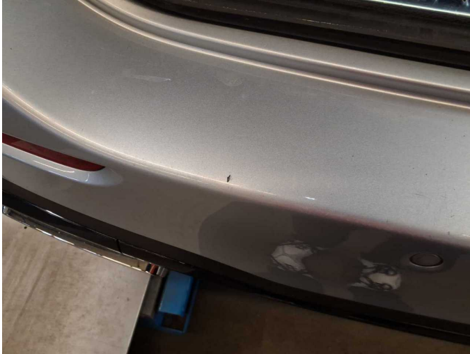
Damage 5: Rear bumper: Rear bumper - Scratch(es) - Paint
