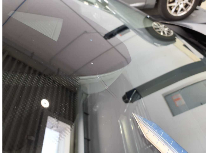
Damage 8: Vehicle glazing: Windscreen - Stone chips - Replace
