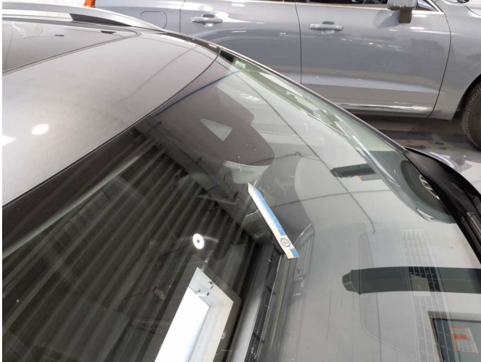
Damage 8: Vehicle glazing: Windscreen - Stone chips - Replace
