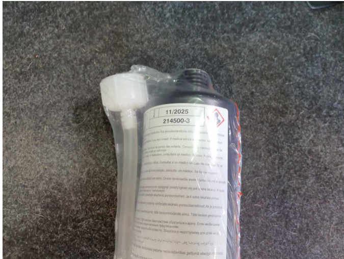
Damage 1: Equipment: Tirefit filler - Expired - Replace
