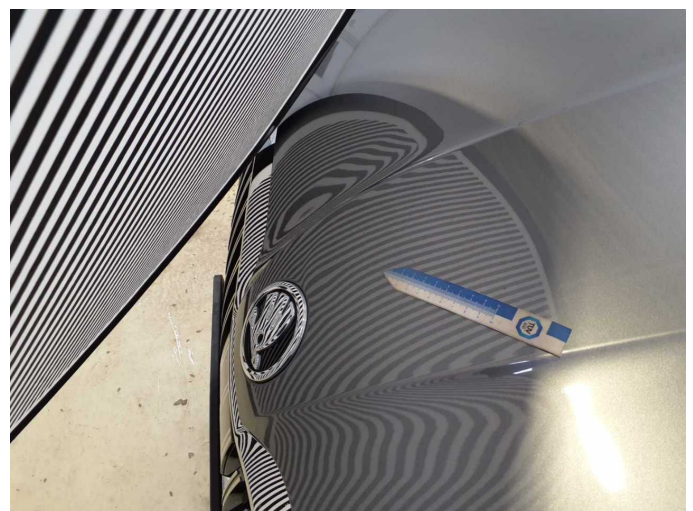
Damage 4: Bonnet: Bonnet - dent(s) - Smooth repair work
