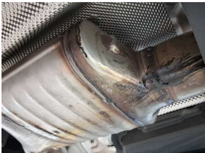
Damage 1: Body: Underbody (Verölt) - Leaking - Perform diagnosis
