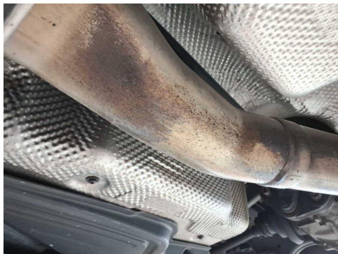
Damage 1: Body: Underbody (Verölt) - Leaking - Perform diagnosis
