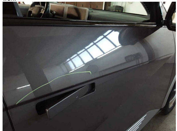
Damage #7: Door - front right side: Door - Scratched - Smart repair
