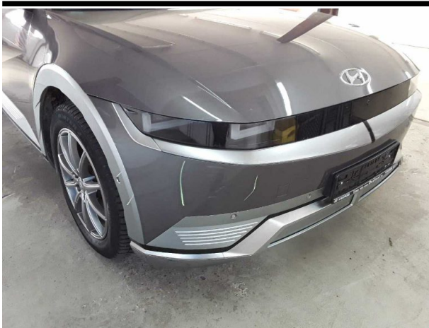
Damage #10: Front bumper: Front bumper - Scratched - Repair and paint
