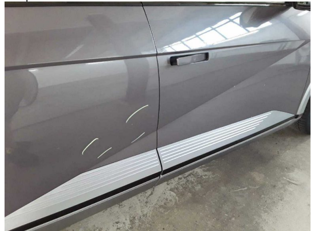
Damage #11: Door - rear right side: Door - Scratched - Repair and paint
