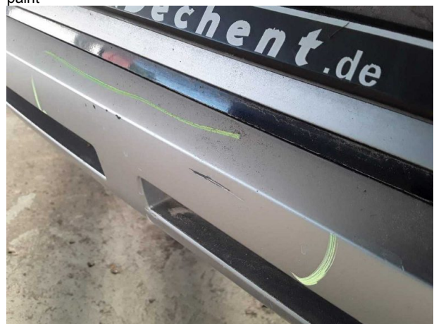
Damage #9: Rear bumper: Spoiler - Scratched - Repair and paint
