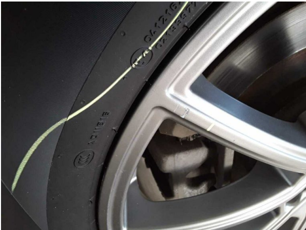
Damage #2: Wheel / tyres: Alloy rim - rear left side - Scratched - ... deduction
