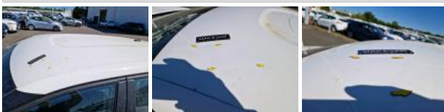
Roof, Dent(s), Repair and paint (complete)
