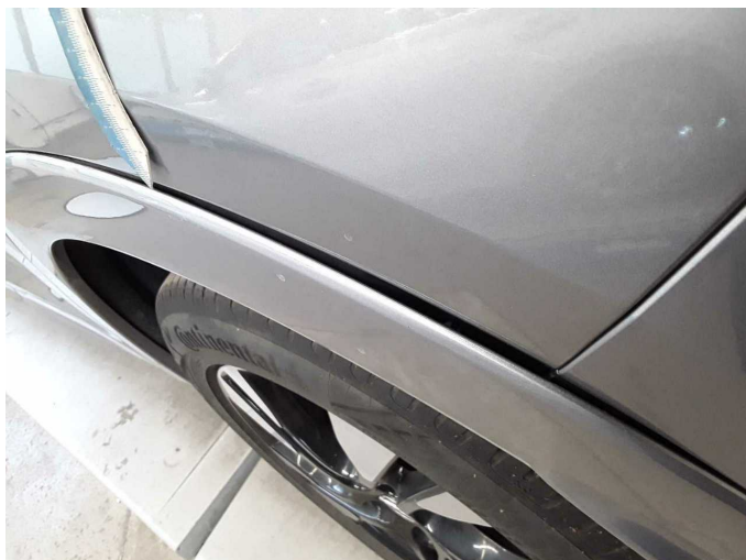
Damage 3: Side panel - rear left side: Wheel arch - Malposition - Un- / install
