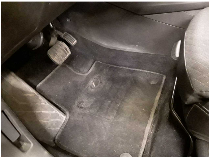
Damage 1: Trim / covers: Floor mats - Damaged - Replace
