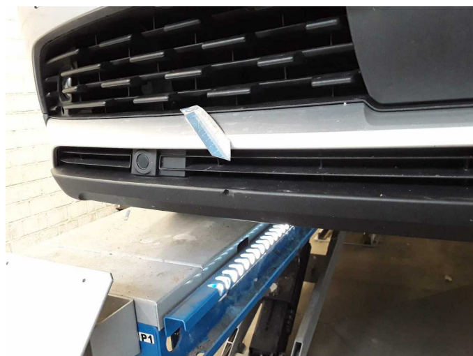
Damage 5: Front bumper: Spoiler - Scratched - Loss in value
