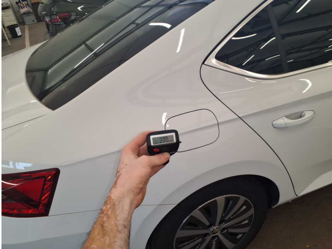
Repainting 1: Side panel - rear right side
