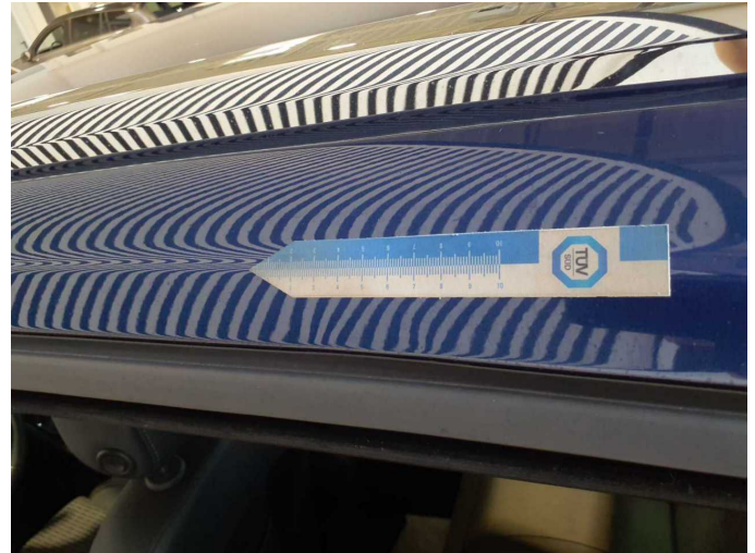
Damage 6: Roof: Roof rail - left side - dent(s) - Smooth repair work
