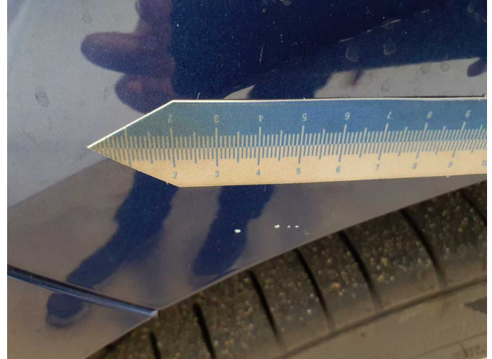
Damage 12: Mudguard - left side: Mudguard - left side - Stone chips - Paint
