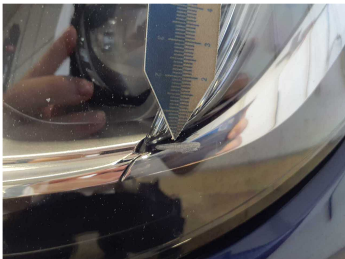
Damage 15: Headlight: Headlight - left side - Broken / torn - repair according to calculation
