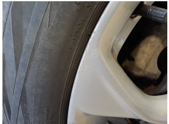
Damage 8: Wheel / tyres: Alloy rim - rear right side - Scratch(es) - Loss in value
