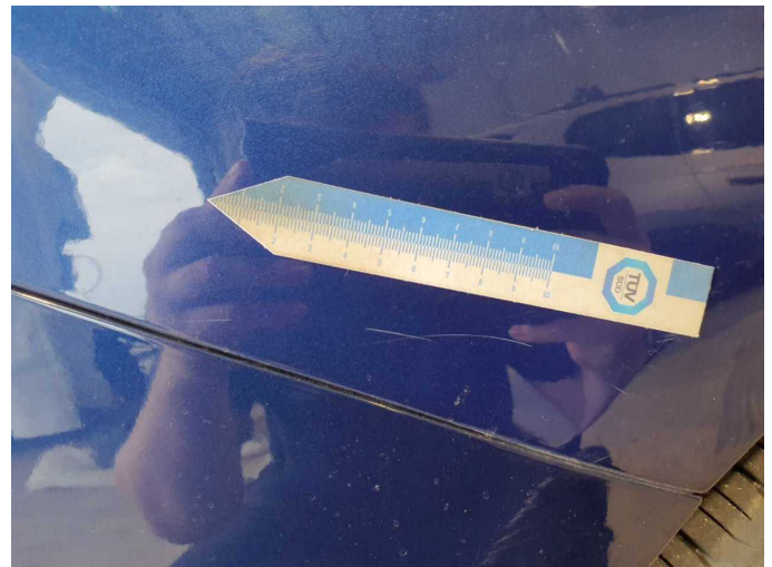
Damage 5: Side panel - rear right side: Side panel - Scratch(es) - Smart repair
