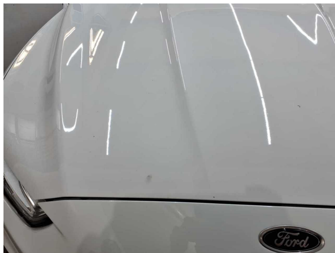
Damage 4: Bonnet: Bonnet - Stone chips - Paint
