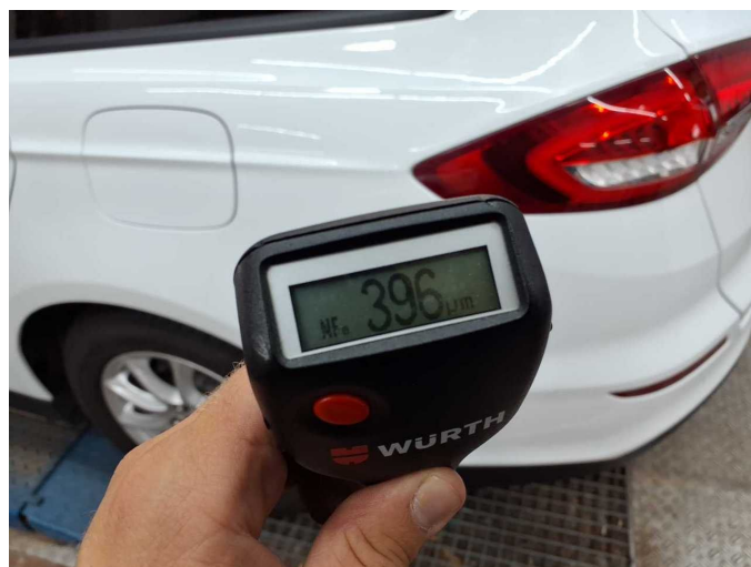
Damage 7: Side panel - rear left side: Side panel (Orangenhaut) - Unprofessionally repaired - Paint
