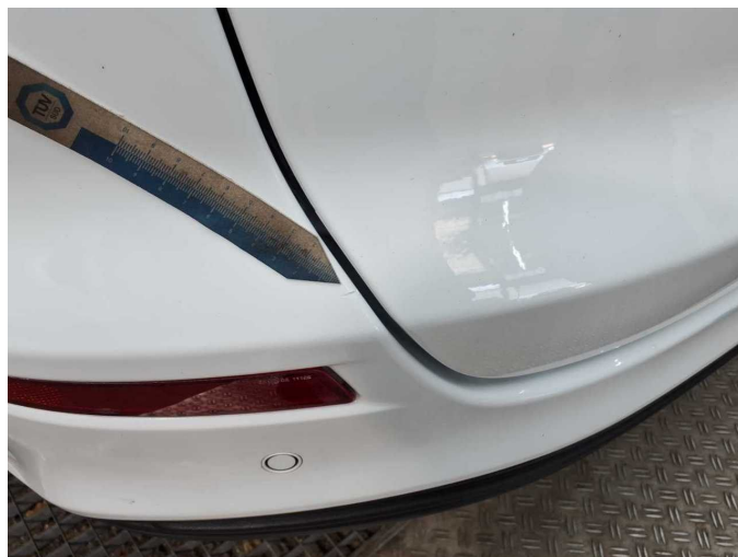
Damage 5: Rear bumper: Rear bumper - Scratch(es) - Paint
