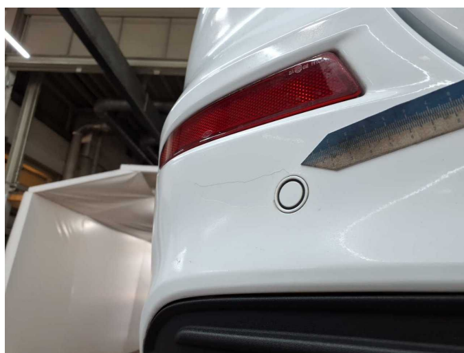
Damage 5: Rear bumper: Rear bumper - Scratch(es) - Paint
