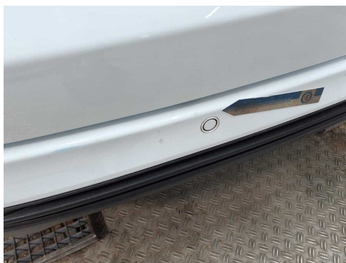
Damage 5: Rear bumper: Rear bumper - Scratch(es) - Paint
