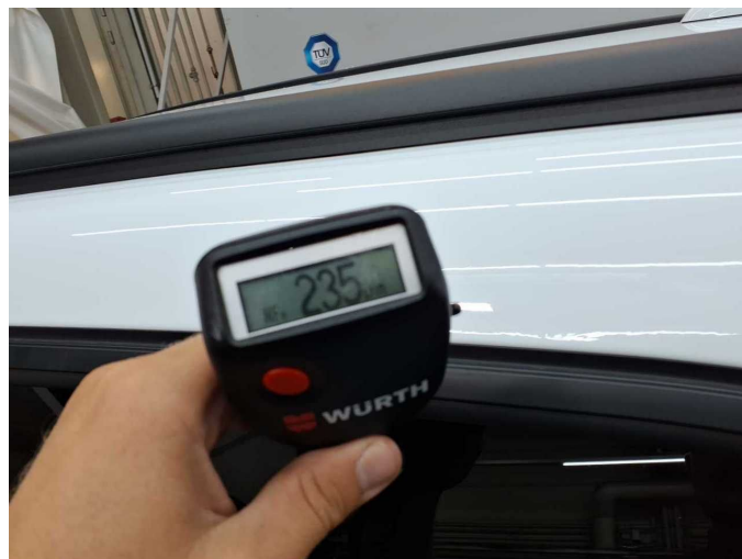
Damage 6: Roof: Roof rail - left side (Orangenhaut.) - Unprofessionally repaired - Paint
