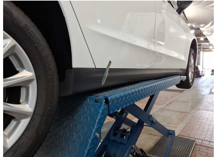
Damage 2: Sill - right side: Trim - Scratch(es) - Loss in value
