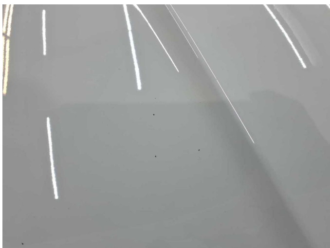
Damage 4: Bonnet: Bonnet - Stone chips - Paint
