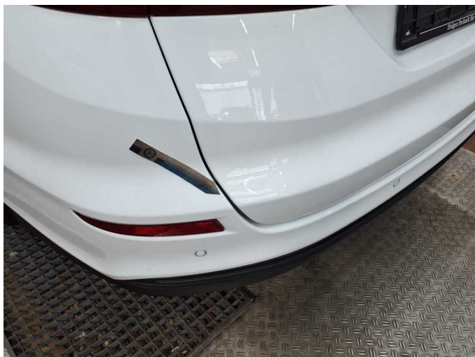
Damage 5: Rear bumper: Rear bumper - Scratch(es) - Paint
