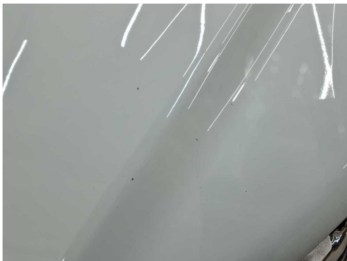
Damage 4: Bonnet: Bonnet - Stone chips - Paint
