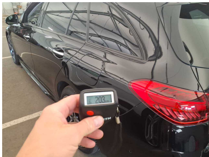
Repainting 1: Side panel - rear left side
