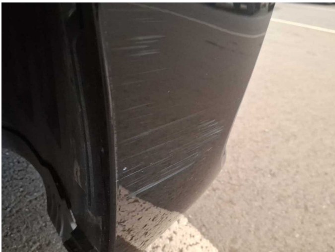
Damage 4: Front bumper: Front bumper - Scratch(es) - Paint
