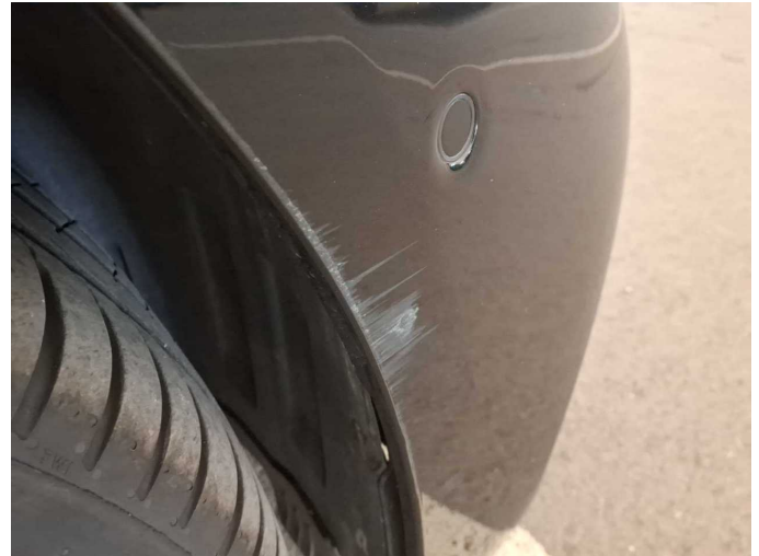
Damage 4: Front bumper: Front bumper - Scratch(es) - Paint
