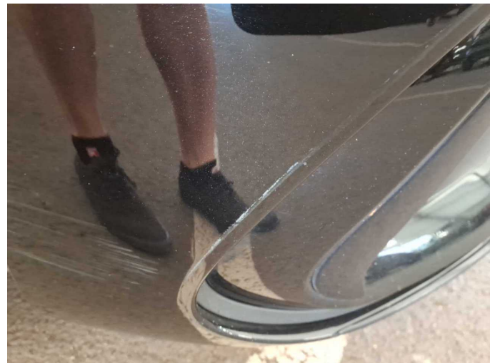
Damage 4: Front bumper: Front bumper - Scratch(es) - Paint
