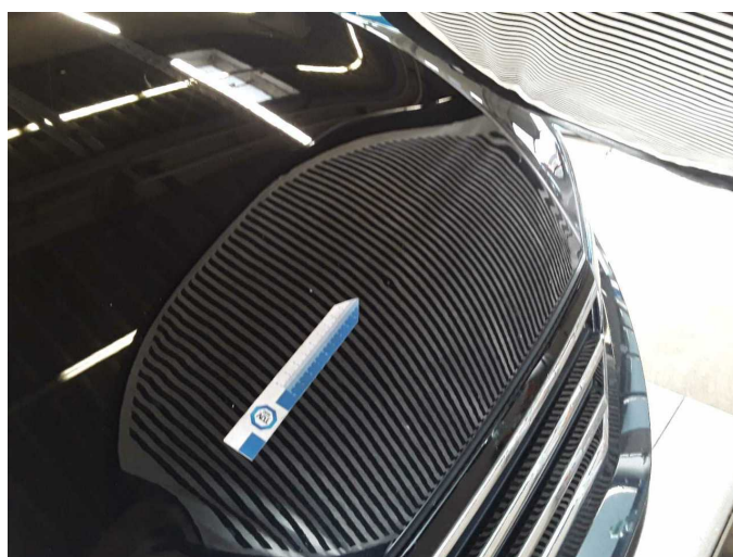
Damage 13: Bonnet: Bonnet - Dent / paintcoat damage - Repair and paint
