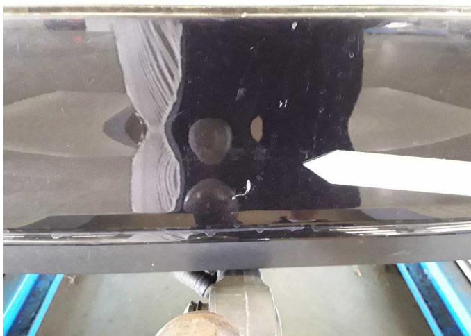
Damage 7: Rear bumper: Rear bumper - Scratched - Paint
