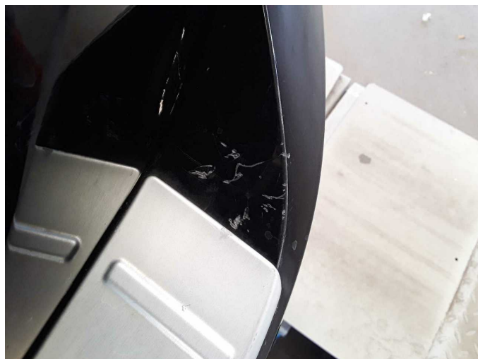
Damage 7: Rear bumper: Rear bumper - Scratched - Paint
