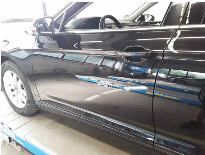
Wear and tear 4: Door - front left side: Door edge - Scratched - Cover / polish
