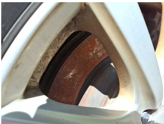
Damage 4: Braking system: Brake discs - rear - Corrosion - Replace
