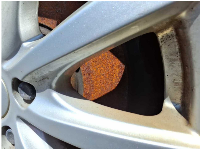
Damage 3: Braking system: Brake discs - front - Corrosion - Replace
