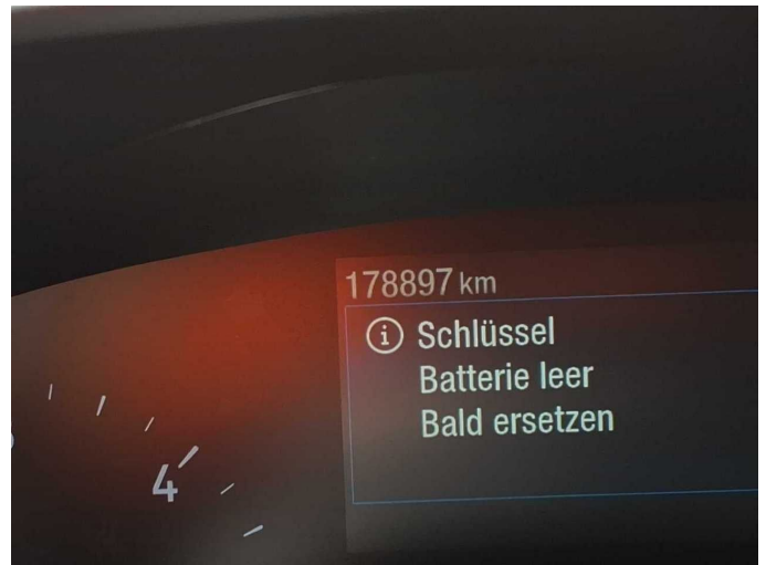
Damage 1: Equipment: Vehicle key (Batterie) - Empty - Replace
