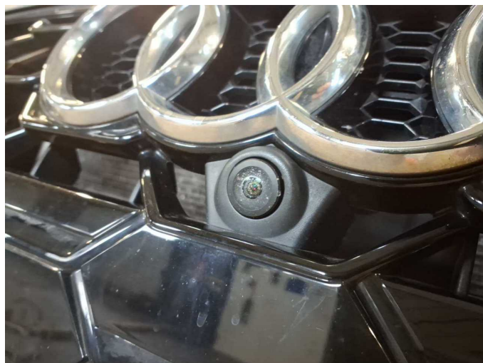
Wear and tear 2: Electronic systems: Front camera - Stone chips - No deduction
