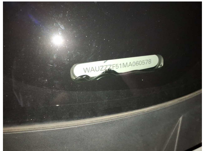
Damage 7: Vehicle glazing: Windscreen (Kleber zu sehen) - Unprofessionally repaired - Un- / install
