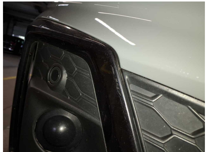
Damage 4: Front bumper: Air-inlet grille (Rechts, Rahmen) - Scratched - Replace
