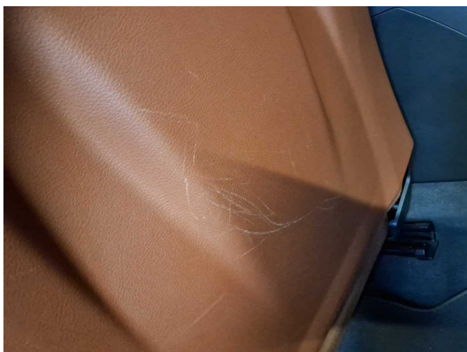
Damage 2: Seat - front: Seat - left side (Abdeckung hinten) - Scratch(es) - Smart repair
