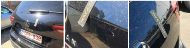
Wing FR, Dent(s), Paintless dent repair
