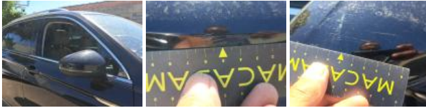
Door FR, Dent(s), Paintless dent repair
