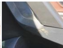
Roof liner, Damaged, Replace
