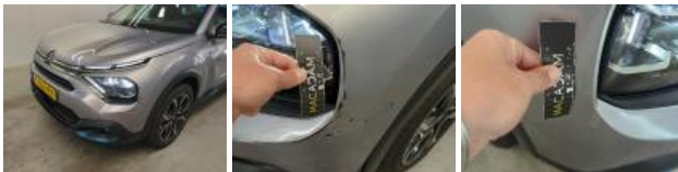
Bumper trim F, Deformed / Strained, Replace
