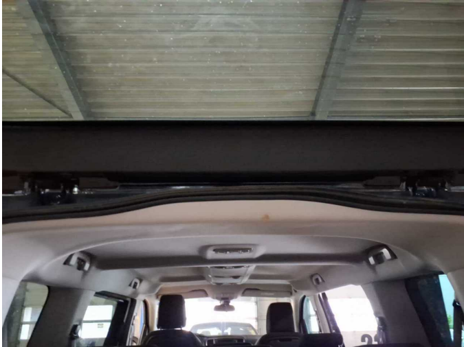
Damage 4: Trim / covers: Roof lining - Soiled - Clean
