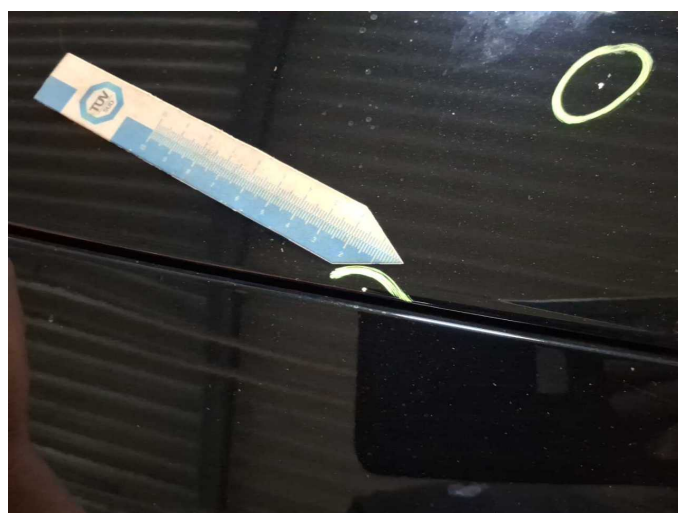
Damage 12: Bonnet: Bonnet - Stone chips - Paint
