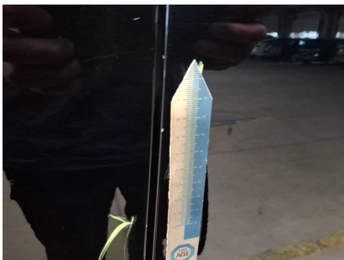
Damage 14: Sliding door - left side: Sliding door - Dent / paintcoat damage - Repair and paint
