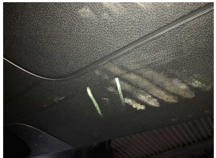
Damage 7: Trim / covers: Boot lid - interior trim - Scratched - Smart repair
