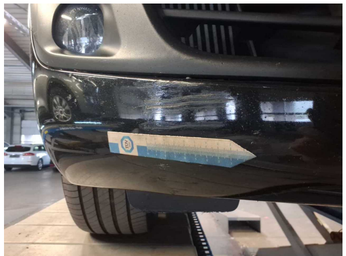
Damage 13: Front bumper: Front bumper (+ Blende) - Scratched - Paint
