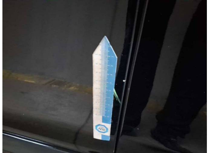
Damage 15: Sliding door, right: Sliding door - Dent / paintcoat damage - Repair and paint
