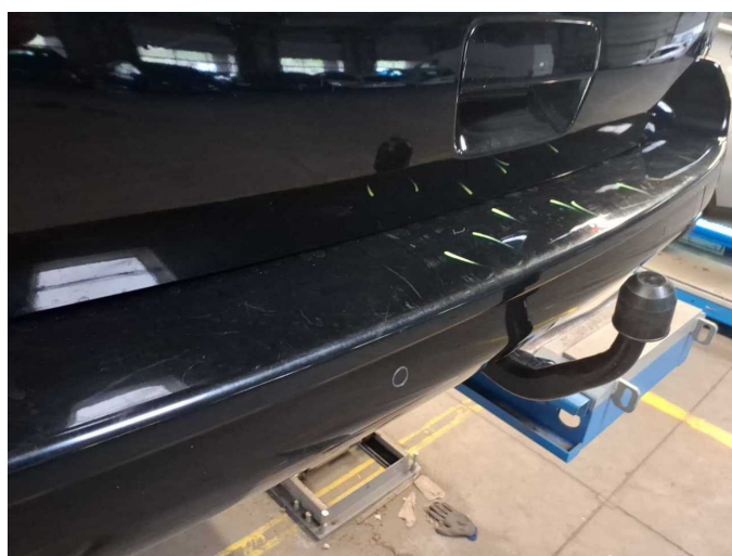
Damage 11: Rear bumper: Rear bumper - Dent / paintcoat damage - Repair and paint
