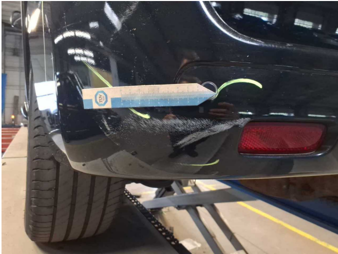
Damage 11: Rear bumper: Rear bumper - Dent / paintcoat damage - Repair and paint
