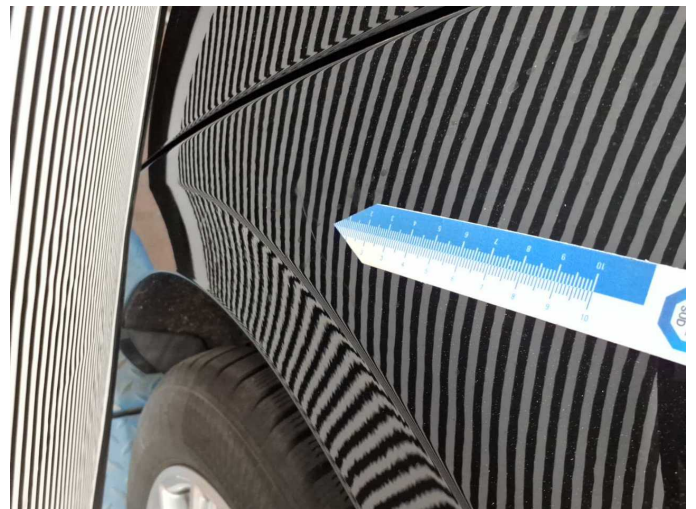
Damage 8: Side panel - rear left side: Side panel - Dent / paintcoat damage - Paint
