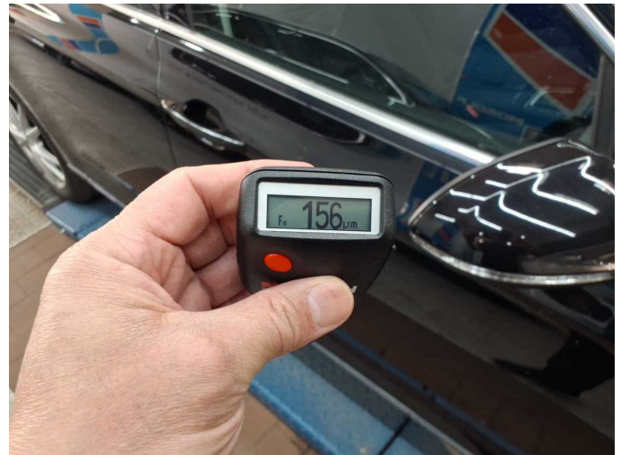
Repainting 1: Roof, Boot lid / rear door, Mudguard - left side, Bonnet, Side panel - rear left side, Side panel - rear right side, Door - front right side
