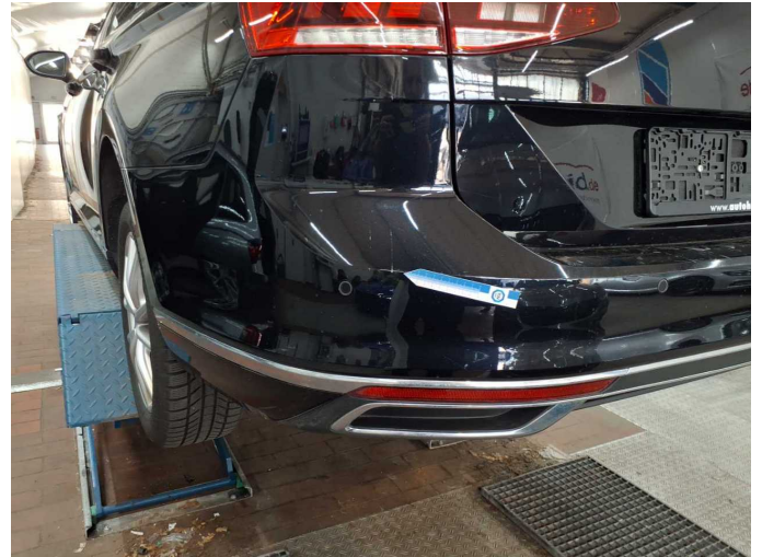
Damage 7: Rear bumper: Rear bumper - Dent / paintcoat damage - Paint
