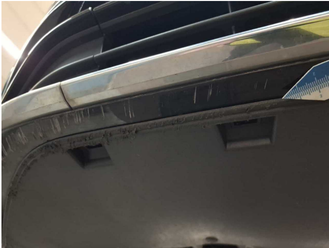
Damage 6: Front bumper: Front bumper (unterhalb) - Scratched - Paint
