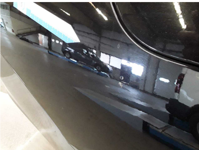
Damage 4: Side panel - rear right side: Side panel (Vogelkot eingebrannt) - Paint defect - Paint
