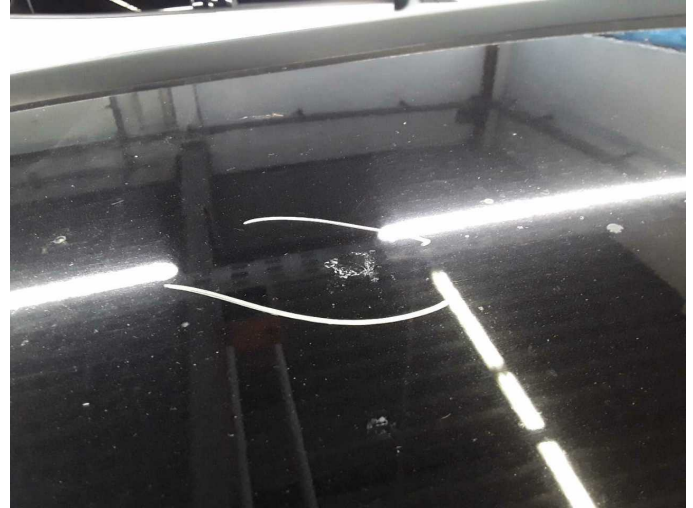
Damage 6: Roof: Roof (Vogelkot eingebrannt) - Paint defect - Paint
