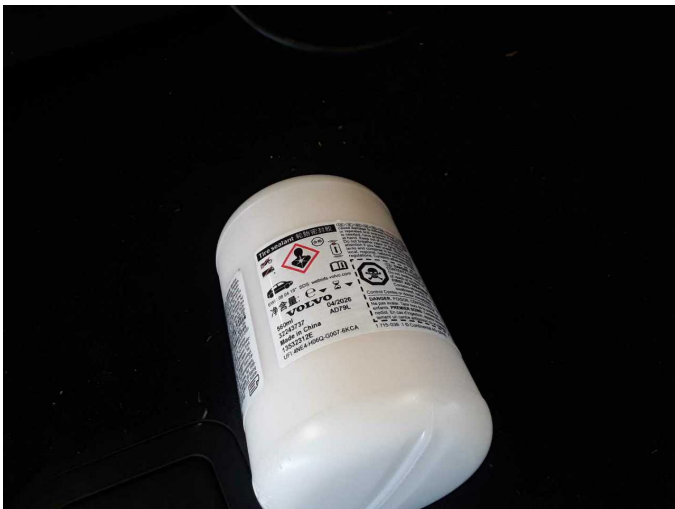
Damage 1: Equipment: Tirefit filler - Expired - Replace
