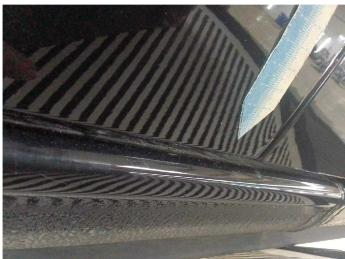
Wear and tear 8: Door - front left side: Door - dent(s) - No deduction
