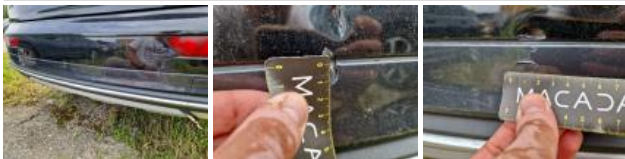
Fog light RL, Broken, Replace
