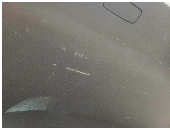
Damage 4: Trim / covers: Boot lid - interior trim - Scratched - Replace
