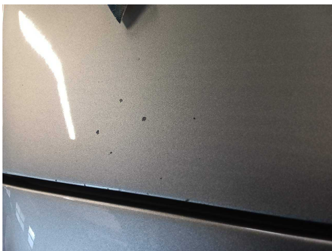
Damage 8: Bonnet: Bonnet - Stone chips - Paint
