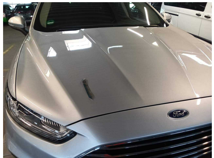
Damage 8: Bonnet: Bonnet - Stone chips - Paint
