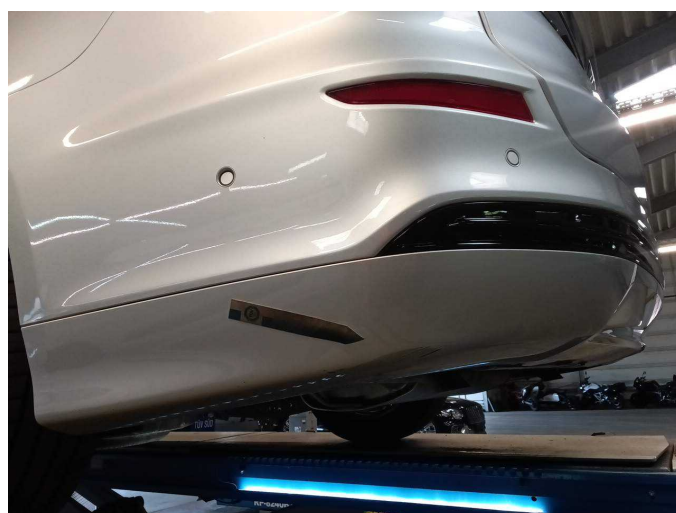
Damage 6: Rear bumper: Spoiler - Scratch(es) - Paint
