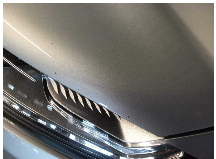
Damage 8: Bonnet: Bonnet - Stone chips - Paint
