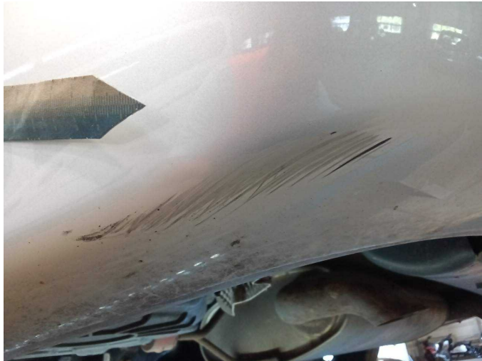
Damage 6: Rear bumper: Spoiler - Scratch(es) - Paint
