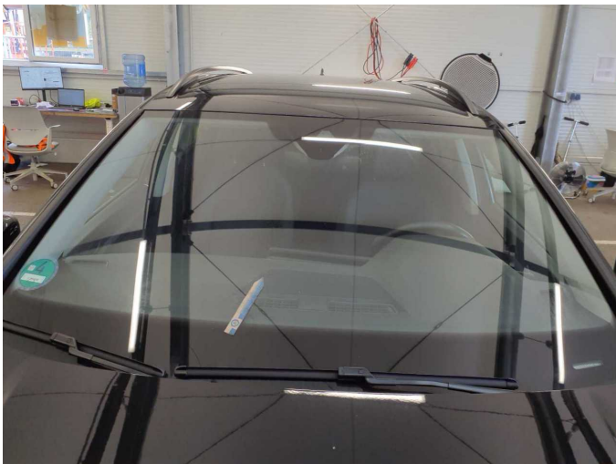
Damage 2: Vehicle glazing: Windscreen with lane departure assistant - Broken / torn - repair according to calculation
