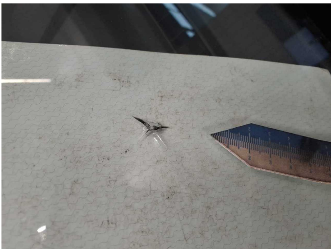
Damage 10: Vehicle glazing: Windscreen (Mit Rissbildung;) - Stone chips - repair according to calculation
