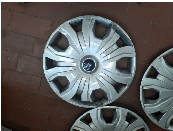
Damage 1: 2nd wheel set: 1 wheel cover - Scratched - Replace
