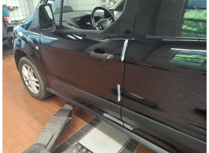
Wear and tear 8: Door - front left side: Door edge - Scratch(es) - Smart repair
