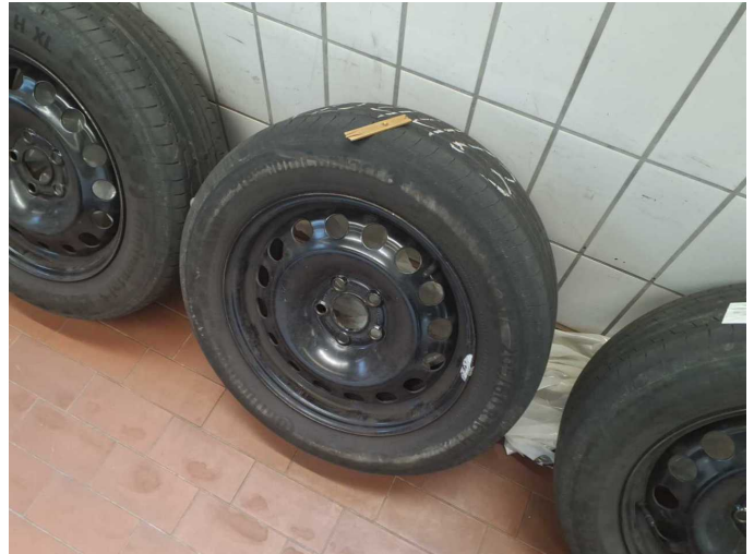
Damage 4: 2nd wheel set: 1 tyre - Worn - Replace
