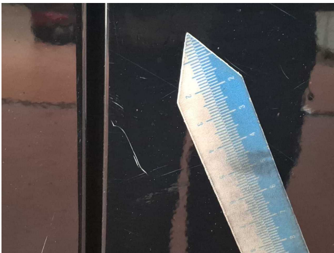
Damage 6: Boot lid / rear door: Rear door - right side - Scratch(es) - Paint
