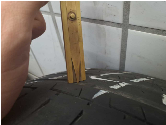
Damage 4: 2nd wheel set: 1 tyre - Worn - Replace
