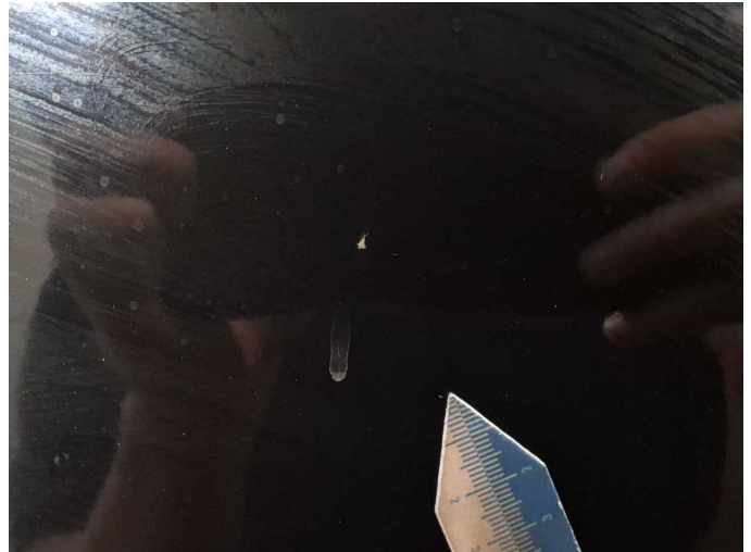
Damage 7: Sliding door, right: Sliding door (Beule) - Dent / paintcoat damage - Repair and paint
