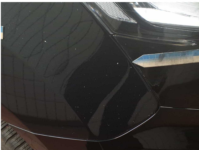
Damage 5: Mudguard - right side: Mudguard - right side (+ Steinschläge) - Scratch(es) - Paint
