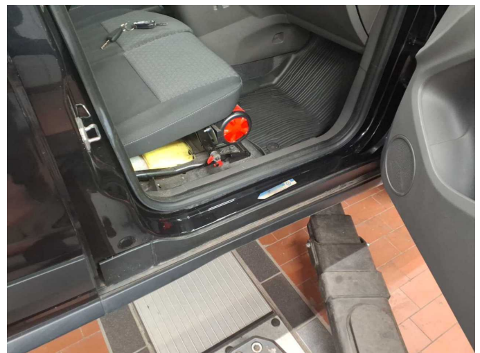
Wear and tear 7: Sill - right side: Sill - dent(s) - No deduction
