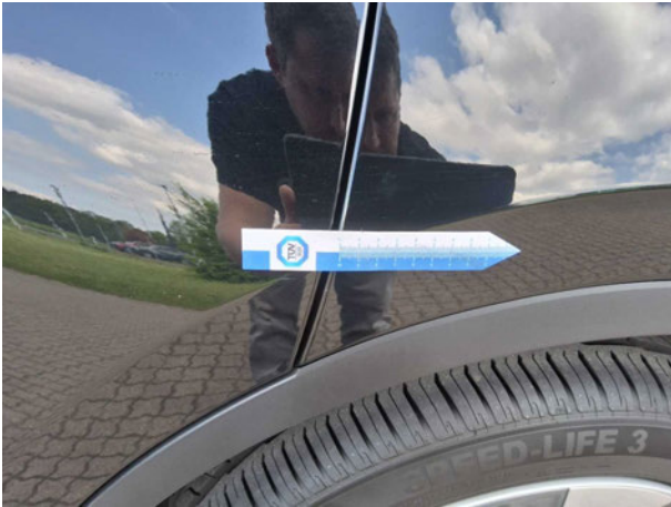
Beschädigung #3: Tür hinten links: Tür - Kratzer - Smart Repair
