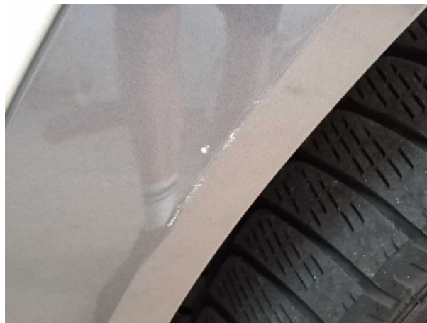
Damage #2: Mudguard - left side: Wheel well extension - Scratched - Replace
