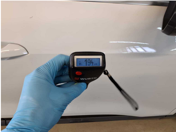
Repainting 1: Door - front right side
