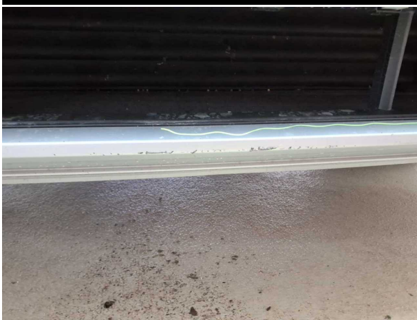
Damage #4: Front bumper: Spoiler - Scratched - Replace
