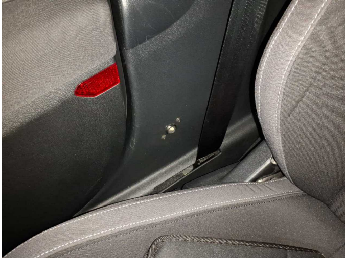
Damage 6: Trim / covers: B-pillar - trim - interior, right side (Fehlbohrung) - Damaged - Replace
