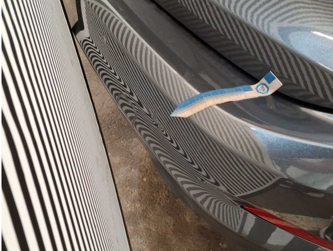
Damage 9: Rear bumper: Rear bumper - Dent / paintcoat damage - Repair and paint
