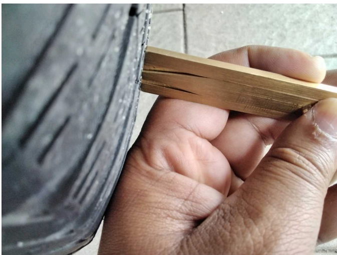
Damage 10: Wheel / tyres: Tyre - right (4mm) - does not meet manufacturer specifications - Replace
