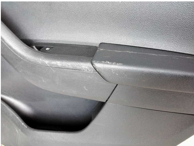
Damage 6: Trim / covers: Door trim - rear right side - Scratch(es) - Loss in value
