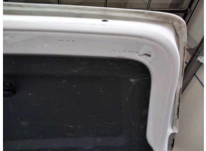
Damage 14: Boot lid / rear door: Boot lid (Innen) - Dent / paintcoat damage - Repair and paint
