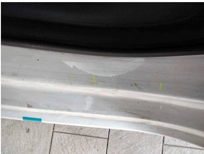
Damage 7: Side panel - rear left side: Sill - Scratch(es) - Smart repair
