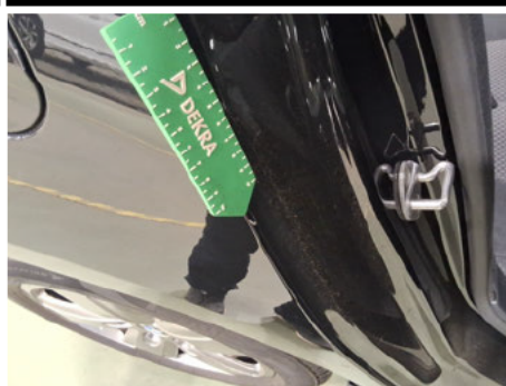
Door sill / Back Right / Scratched
