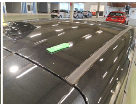
Roof / - / Paint etching
