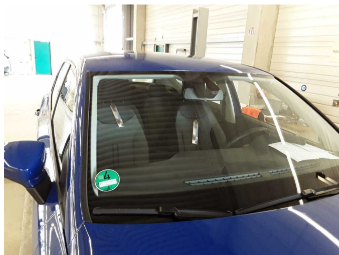
Damage 4: Vehicle glazing: Windscreen with rain sensor - Stone chips - Replace
