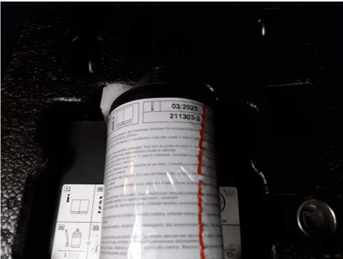
Damage 1: Equipment: Tirefit filler - Expired - Replace
